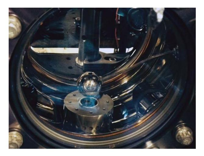
The vacuum chamber of the atom interferometer. Credit: Holger Muller photo., CC BY
