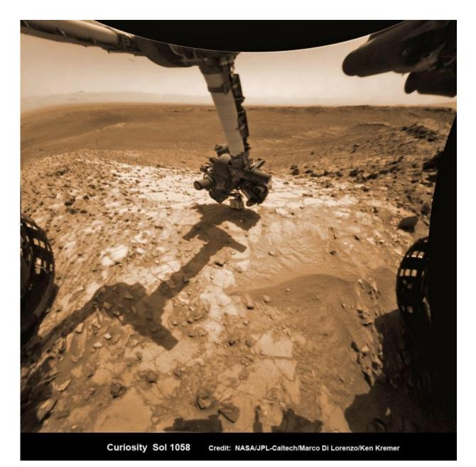
NASA Curiosity rover inspects 'Buckskin' rock outcrop on Mars with APXS mineral spectrometer in this hazcam camera raw image taken on July 29, 2015 (Sol 1058), colorized and linearized. Credit: NASA/JPL-Caltech/Marco Di Lorenzo/Ken Kremer/kenkremer.com
