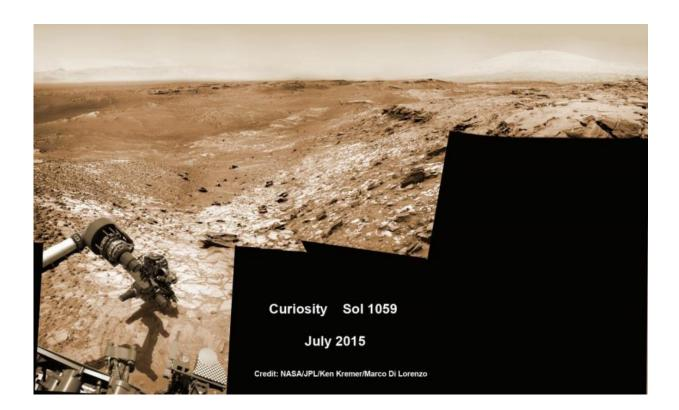
Curiosity extends robotic arm and conducts test drill at "Buckskin" rock target at bright toned "Lion" outcrop on the lower region of Mount Sharp on Mars, seen at right. Gale Crater eroded rim seen in the distant background at left, in this composite multisol mosaic of navcam raw images taken to Sol 1059, July 30, 2015. Navcam camera raw images stitched and colorized. Credit: NASA/JPL-Caltech/Ken Kremer/kenkremer.com/Marco Di Lorenzo
