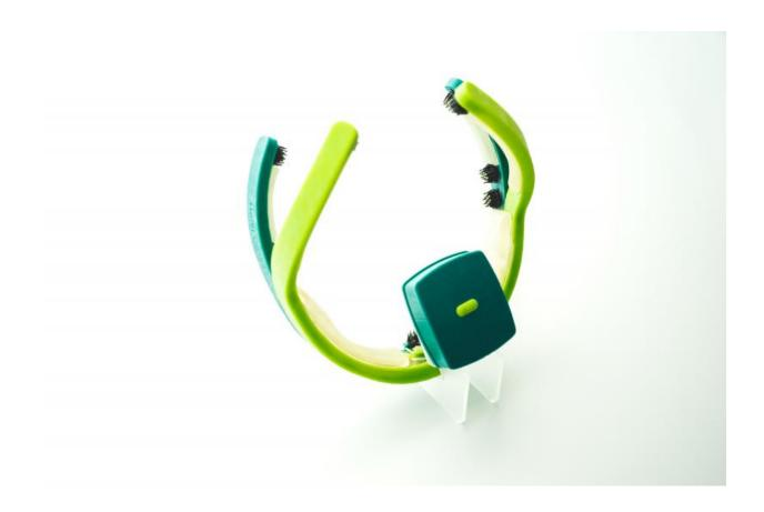
Comfortable EEG headset developed by imec and Holst Centre. The headset enables effective brain-computer interfacing and can monitor emotions and mood in daily life situations using a smartphone application.
