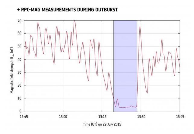
The decrease in magnetic field strength measured by Rosetta's RPC-MAG instrument during the outburst event on 29 July 2015. This is the first time a 'diamagnetic cavity' has been detected at Comet 67P/Churyumov–Gerasimenko
