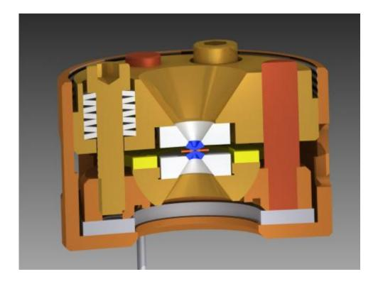
This cutaway schematic shows the diamond anvil cell, a pressure vessel in which the experiments were conducted. The target material is situated between two diamonds, represented here in blue. For this study, a diamond anvil generated pressures to 100,000 times sea level. Credit: University of Chicago/Argonne National Laboratory
