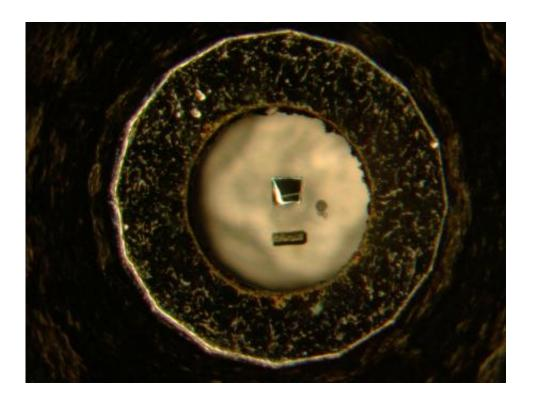
One of the metallic samples studied, niobium diselenide, is seen here-the square in the center-as prepared for an X-ray diffraction experiment. Credit: University of Chicago/Argonne National Laboratory
