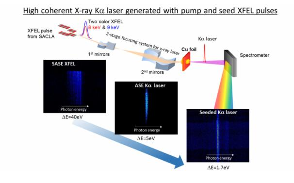
Using copper foil as a medium bombarded by two X-ray pulses of different energies produced by an X-ray free-electron laser, researchers at the University of Electro-Communications in Tokyo have successfully created a powerful and highly coherent atomic X-ray laser with the shortest wavelength to date.
