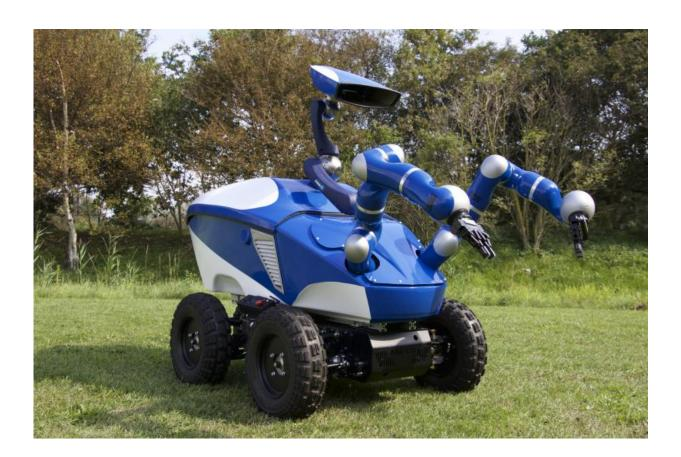
ESA's Interact Centaur rover, developed for telerobotics experiments. The 4x4 wheeled vehicle combines a camera head on a neck system, a pair of highly advanced force sensitive robotic arms designed for remote force-feedback-based operation and a number of proximity and localisation sensors. Credit: ESA
