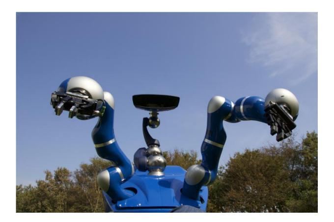
ESA's Interact Centaur rover has a pair of robotic arms that can flex in a similar manner to human arms and can provide the operator with force feedback to let them know the robot has encountered an obstacle but not damaged anything. Credit: ESA
