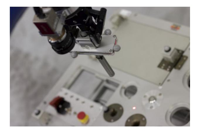
The 'operations task board' that ESA's Interact Centaur rover, controlled from the ISS by Andreas Mogensen, will locate and then then to remove and plug a metal pin into. The pin has a very tight mechanical fit and tolerance of only about 150 micrometres, less than a sixth of a millimetre. Credit: ESA
