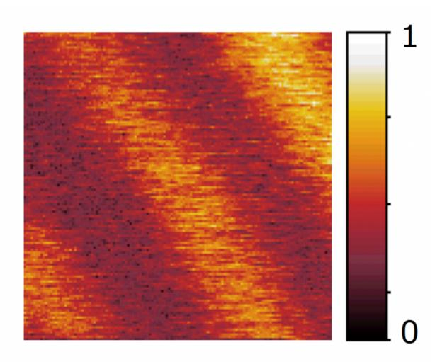
Studying a known thin-layer sample using the novel nanoscope. Laser pulses excite the electrons in the bright stripes, whereby the otherwise transparent
