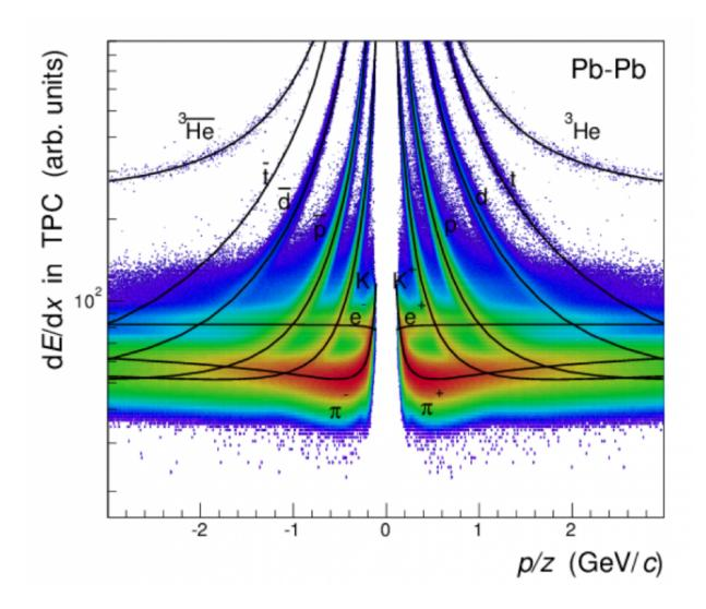
Measurements of energy loss in the time-projection chamber enable the ALICE experiment to identify antinuclei (upper curves on the left) and nuclei (upper
