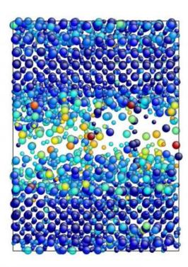
This computer-generated image shows how atomic scale blending of ceramic materials can distort crystal structures of the blended ceramics during mechanical stretch. It's being tested in Ashfaq Adnan's research. Credit: UT Arlington
