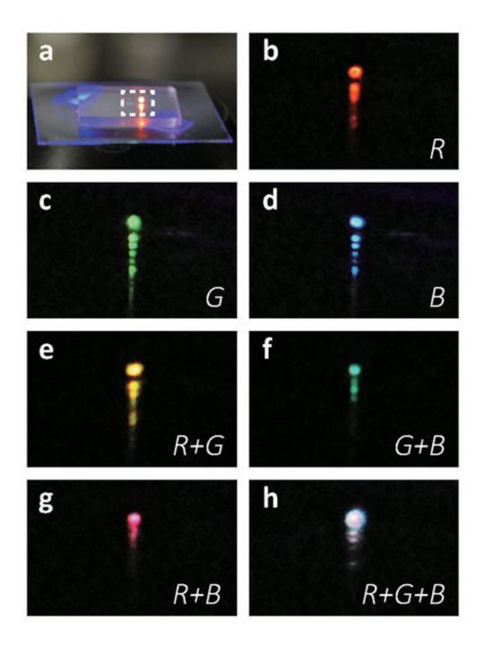
This photo collage, supplied by the researchers, shows the mixed emission color from a multi-segment nanosheet in the colors of red, green, blue, yellow, cyan, magenta and white. The top dots in each photograph are the direct image of laser emission, while the tails under these dots are the reflection from the substrate. Credit: ASU/*Nature Nanotechnology*
