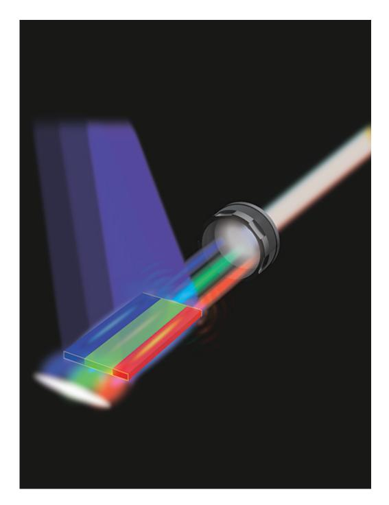
This schematic illustrates the novel nanosheet with three parallel segments created by the researchers, each supporting laser action in one of three elementary colors. The device is capable of lasing in any visible color, completely tunable from red, green to blue, or any color in between. When the total field is collected, a white color emerges. Credit: ASU/Nature Nanotechnology
