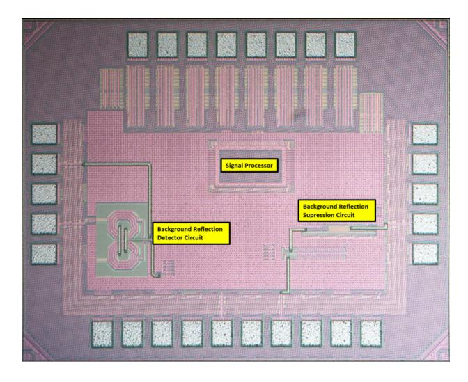
The microchip for wearable devices developed by researchers at JPL and UCLA reflects wireless signals instead of using regular transmitters and receivers. Credit: JPL-Caltech/UCLA
