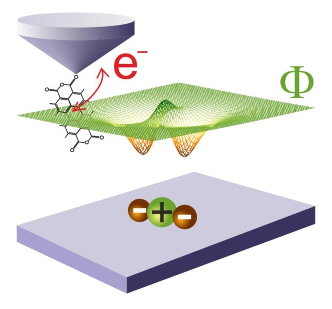
Illustration of the measuring principle: depending on the local electric potential field of a nanostructure on the surface of a sample, a single electron jumps from the tip of the microscope to the sensor molecule or back. Credit: Forschungszentrum Jülich
