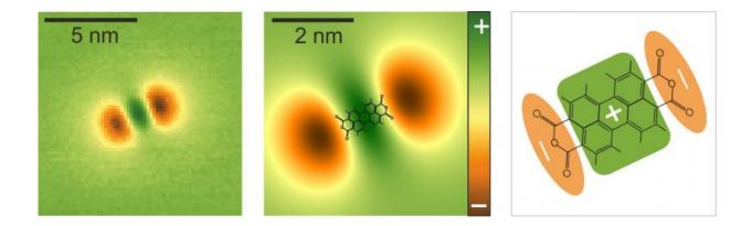
Left: The scanning quantum dot micrograph of a PTCDA molecule reveals the negative partial charges at the ends of the molecule as well as the positive partial charges in the centre. Centre: Simulated electric potential above a PTCDA molecule with molecular structure Right: Schematic of charge distribution in the PTCDA molecule. Credit: Forschungszentrum Jülich
