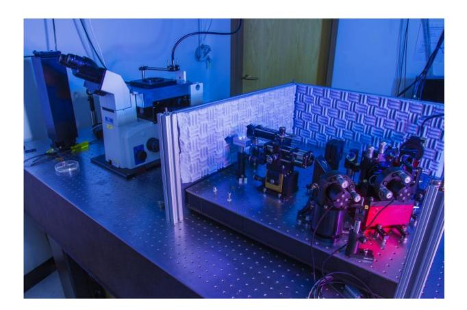
JILA instrument for accurately tracking microscopic objects such as DNA molecules for many hours. The microscope is on the left. The sample is mounted on the black block on top of the silver stage. The lasers and optics are on the right. Credit: Burrus/NIST
