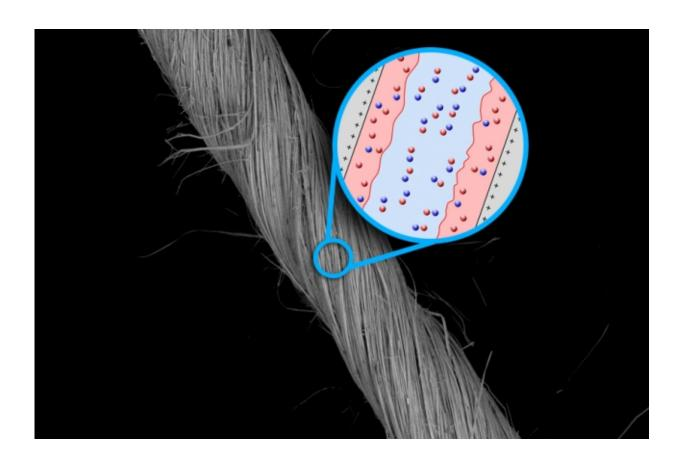
Yarn made of niobium nanowires, seen here in a scanning electron microscope image (background), can be used to make very efficient supercapacitors, MIT researchers have found. Adding a coating of a conductive polymer to the yarn (shown in pink, inset) further increases the capacitor's charge capacity. Positive and negative ions in the material are depicted as blue and red spheres.
