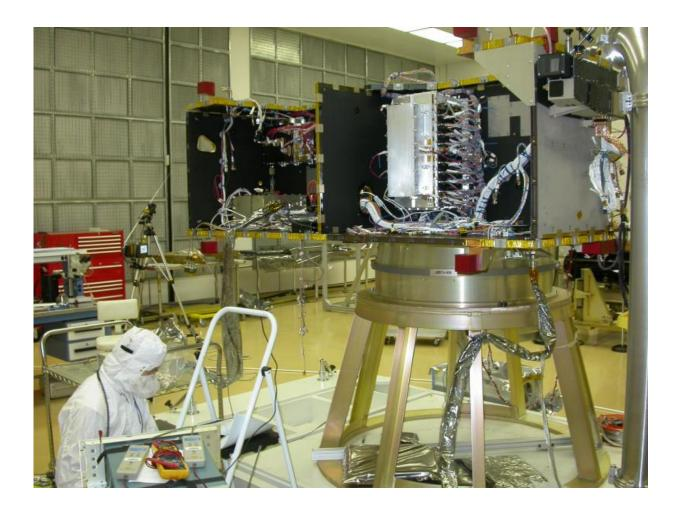
Checking New Horizons' electronics, pre-launch. Credit: NASA/JHUAPL/SwRI, CC BY
