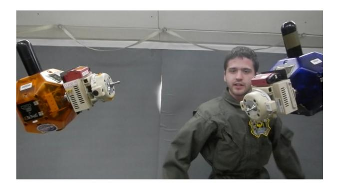
MIT's Lennon Rodgers, a research scientist who did graduate work in the MIT Space Systems Laboratory (SSL), led a team of students to build a universal docking port (UDP) for the <u>Synchronized Position Hold</u>, <u>Engage, Reorient Experimental Satellites (SPHERES</u>) testbed on the International Space Station (ISS). The flight versions were subsequently developed by graduate students Duncan Miller, David Sternberg, and
