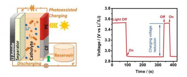
(Left) Illustration of the new Li-I solar flow battery with an aqueous electrolyte, which compared to organic solvents has advantages in terms of performance, cost, and environmental friendliness. (Right) When the solar battery is exposed to light, the voltage that it needs from an external source immediately decreases, as the device is being charged by the solar cell. Credit: Yu, et al. ©2015 American Chemical Society
