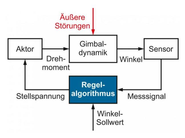
The optimized control algorithm calculates thousands of measurements per seconds, including vibrations of the aircraft, and stabilizes the image. Credit: TU Wien
