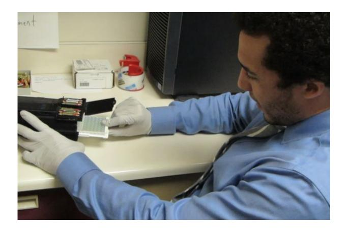
The new ELISA platform is created with a 3D printer and attaches to a smartphone.
