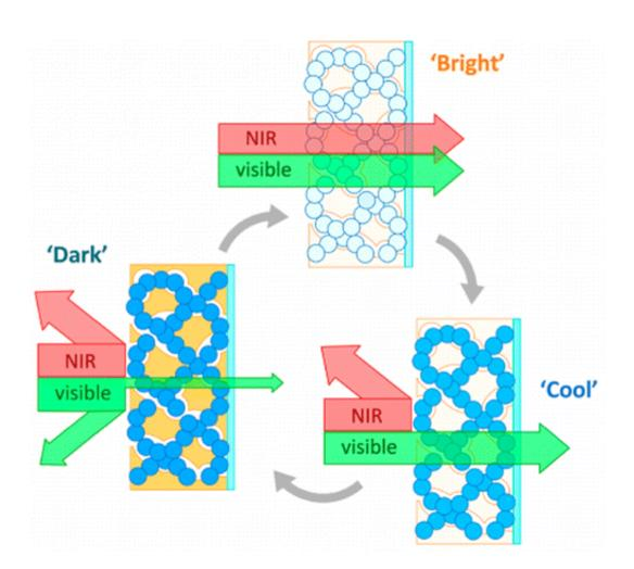
The illustration demonstrates the dark, bright and cool mode made possible by the researchers' new architected nanocomposite. The team organized the two components of the composite material to create a porous interpenetrating network. This organization enables substantially faster switching between modes. Credit: Cockrell School of Engineering
