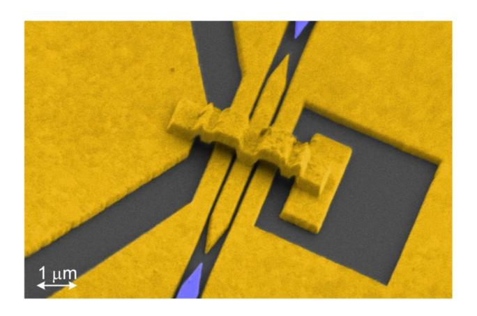
A colorized electron microscope image of a micro-modulator made of gold. In the slit in the center of the picture light is converted into plasmon polaritons, modulated and then re-converted into light pulses. Credit: Haffner et al. *Nature Photonics* 2015
