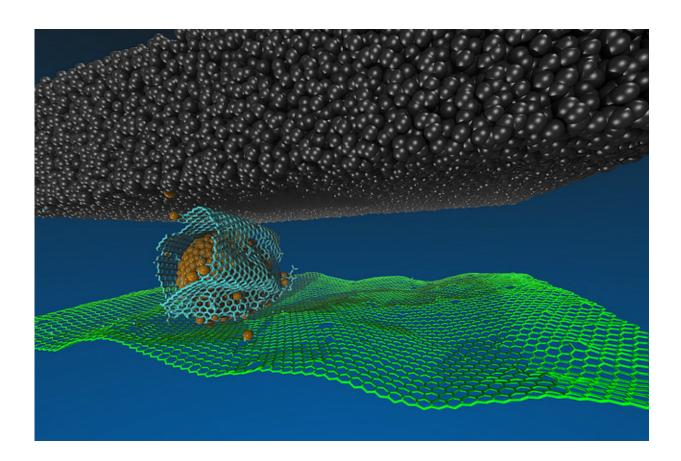
In this schematic of the superlubricity system, the gold represents nanodiamond particles; the blue is a graphene nanoscroll; green shows underlying graphene on silicon dioxide; and the black structures are the diamond-like carbon interface. Credit: Sanket Deshmukh, Joseph Insley, and Subramanian Sankaranarayanan, Argonne National Laboratory
