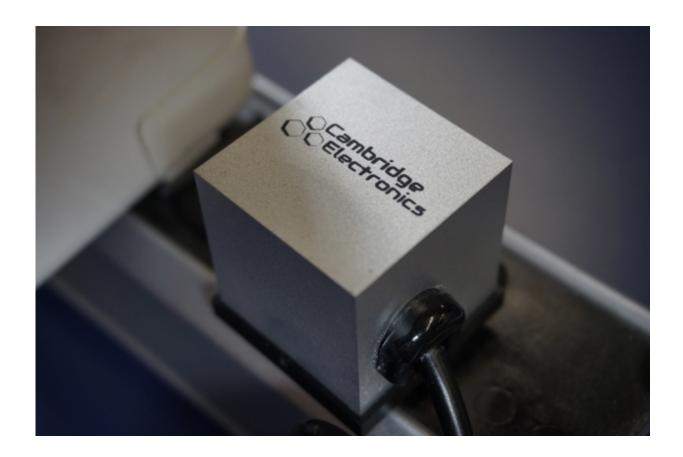
Shown here is a prototype laptop power adapter made by Cambridge Electronics using GaN transistors. At 1.5 cubic inches, this is the smallest laptop power adapter ever made. Credit: Cambridge Electronics
