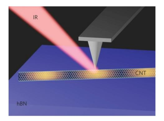
Illustration of s-SNOM shows Infrared (IR) light focused onto AFM tip to excite plasmons in a carbon nanotube (CNT) on a boron nitride (BN) substrate.
