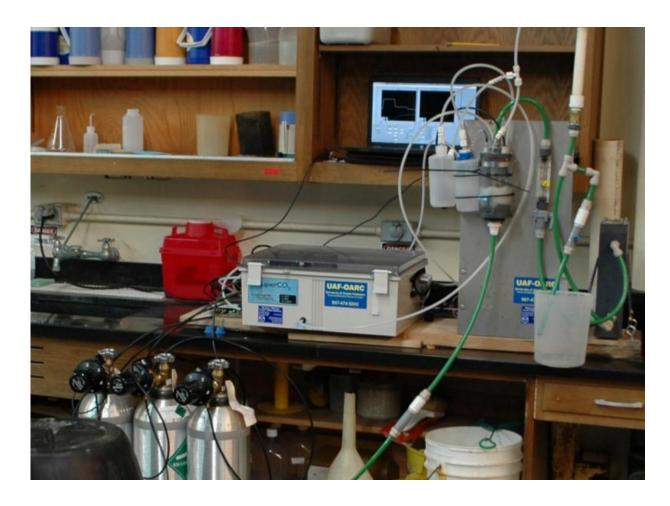
This system, called a Burkolator because it was developed by Burke Hales at Oregon State University, measures carbon dioxide in seawater to help monitor ocean acidification. Credit: Wiley Evans/ NOAA
