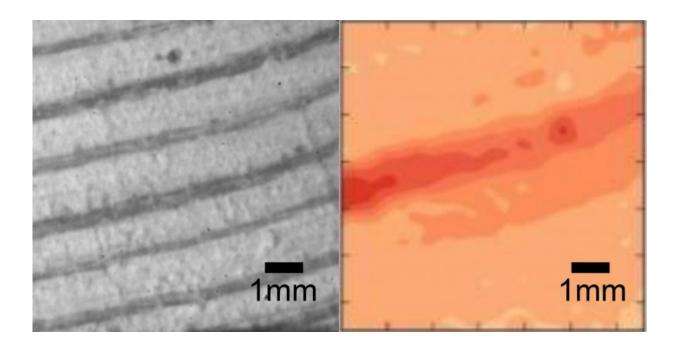
Year rings show collapse as a result of the piston's compression. The images taken by the camera clearly display the year rings of the wood. Comparing two consecutive images reveals the collapse of a year ring. This is seen in the picture on the right as a dark red stripe, which signifies a large local deformation. Credit: Markus Ovaska
