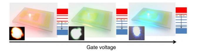
The graphene-based LED's color depends on the applied voltage. The red and blue diagrams show electrons excited to different energy levels, corresponding to different photon energies and therefore different colors of light emission. Credit: Wang, et al. ©2015 Nature
