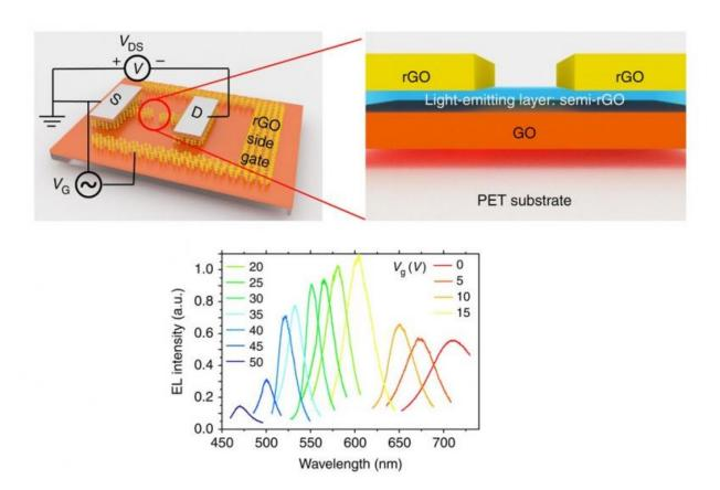
(Top) The light-emitting layer lies at the interface between graphene oxide (GO) and reduced graphene oxide (rGO). (Bottom) Typical electroluminescent spectra of a single graphene-based LED. Credit: Wang, et al. ©2015 Nature
