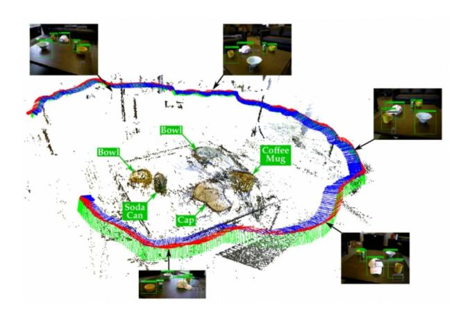
The proposed SLAM-aware object recognition system is able to localize and recognize several objects in the scene, aggregating detection evidence across multiple views. The annotations are actual predictions proposed by the system.
