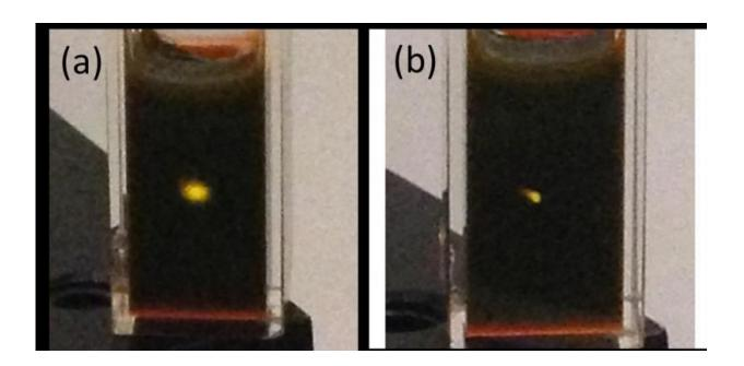
Photographs of upconversion in a cuvette containing cadmium selenide/rubrene mixture. The yellow spot is emission from the rubrene originating from (a) an unfocused continuous wave 800 nm laser with an intensity of 300 W/cm2. (b) a focused continuous wave 980 nm laser with an intensity of 2000 W/cm2. The photographs, taken with an iPhone 5, were not modified in any way. Credit: Zhiyuan Huang, UC Riverside.
