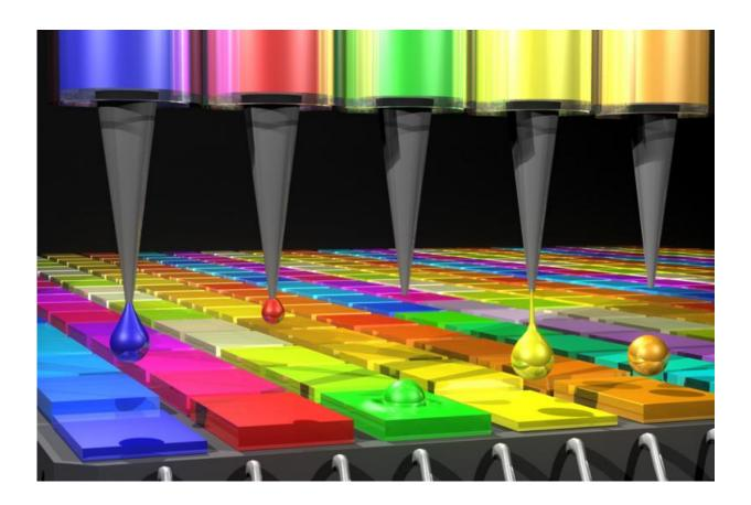
In this illustration, the Quantum Dot (QD) spectrometer device is printing QD filters — a key fabrication step. Other spectrometer approaches have complicated systems in order to create the optical structures needed. Here in the QD spectrometer approach, the optical structure — QD filters — are generated by printing liquid droplets. This approach is unique and advantageous in terms of flexibility, simplicity, and cost reduction.
