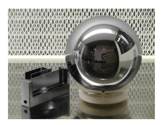
The number of atoms in this silicon sphere is known given or taken 20 atoms each 10^9. The atom distance was measured by the X-ray interferometer on the left. Credit: Enrico Massa and Carlo Sasso
