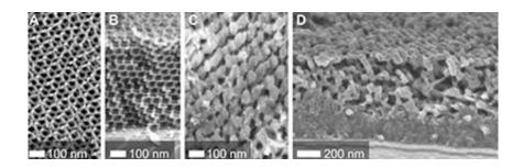
Scanning electron microscopy micrographs show a periodically ordered mesoporous gyroidal resin template (A and B) and the resulting laser-induced crystalline silicon nanostructure after template removal (C and D). Credit: Cornell University
