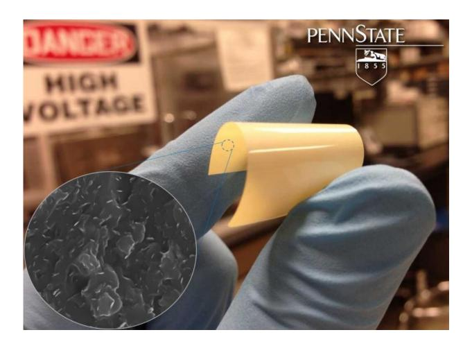
Flexible polymer nanocomposite thin films for high-temperature high-voltage capacitive energy storage. Credit: Q. Li
