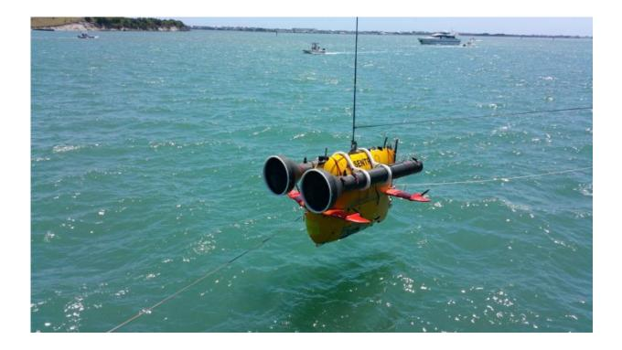
The robot submarine named Sentry, equipped with the SyPRID samplers, being lowered into the water from the RV Atlantis. Credit: Andrew Billings, WHOI
