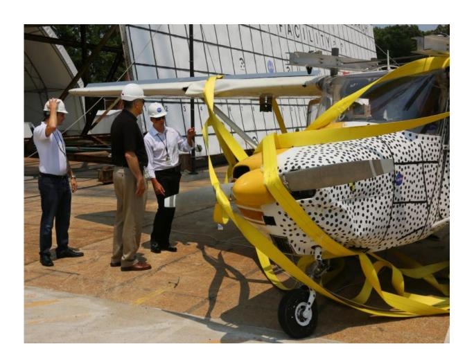
The crash test simulated a controlled emergency landing on a highway or runway. Technicians had to set up a large yellow net to keep the plane from going into a pool that is used for spacecraft water impact testing. Credit: NASA Langley/David C. Bowman
