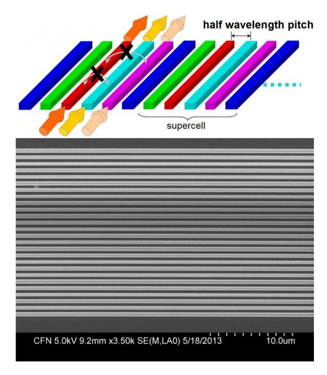
High-density silicon waveguides (26 shown) that have a half-wavelength pitch (a=780nm for  $\lambda$ =1550nm) and fill 50% of the surface area of the underlying substrate have been engineered to achieve inter-waveguide crosstalk below -20dB, paving the way for high-density integrated optical chips.
