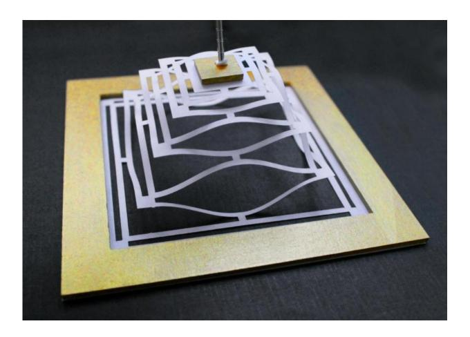
A paper model of a kirigami out-of-plane spring. Credit: McEuen lab
