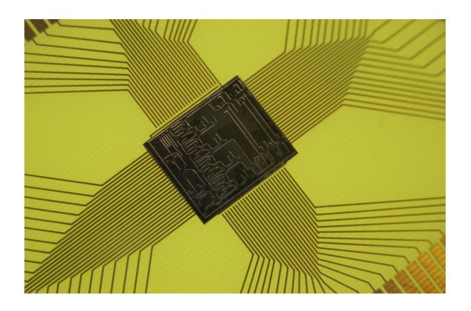
Lab-on-a-chip microfluidic devices can manipulate liquids at ever smaller scales. Credit: Atdr gs/Wikimedia Commons, CC BY-SA
