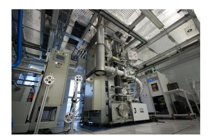
Silica fibre drawing tower in the Zepler Institute Cleanroom Complex.
