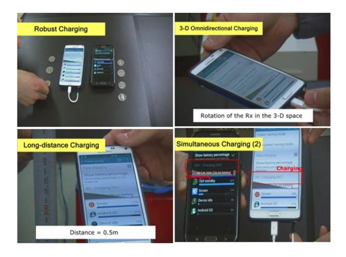
A demonstration of the omnidirectional wireless-charging system (clockwise from top of the left, robust charging despite the presence of metal obstacles,
