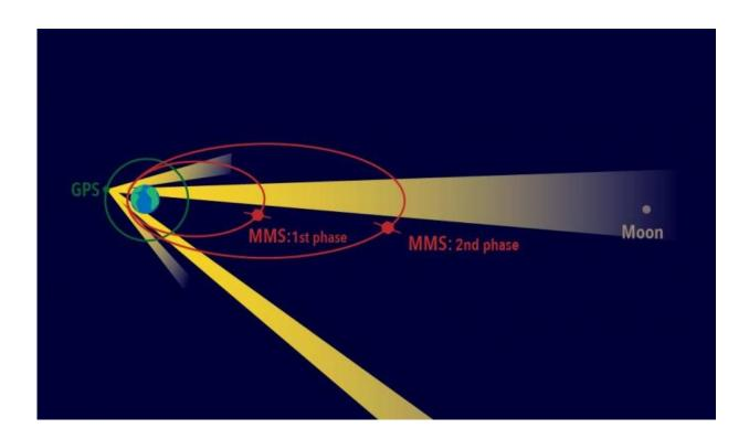
This diagram of MMS orbits for different phases compared to orbits of GPS satellites shows the unique way MMS uses GPS. Because MMS flies above the orbit of GPS satellites, the MMS spacecraft receive their GPS signals from the opposite side of Earth. Credit: NASA
