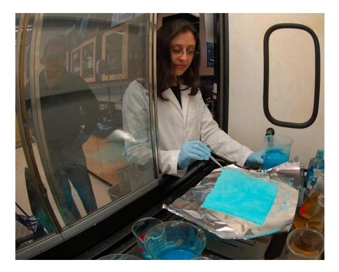
Marcia Silva da Pinto, post-doctoral researcher, works on growing metal organic frameworks onto cotton samples to create a filtration system capable of capturing toxic gas, as Juan Hinestroza looks on. Credit: Mark Vorreuter/File Photo
