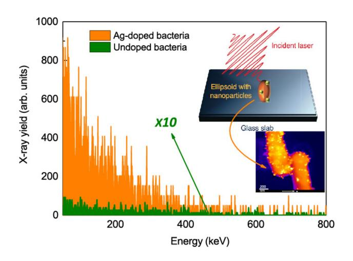
A 10,000 fold enhanced X-ray emission from nanoparticle doped bacteria, from plasma generated by intense ultra short infrared pulses. Credit: Tata Institute of Fundamental Research
