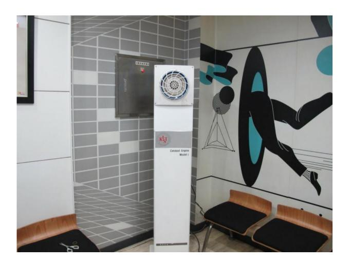
A prototype of the air cleaning equipment for cigarette smoke installed in an actual smoking room. Credit: ©KIST
