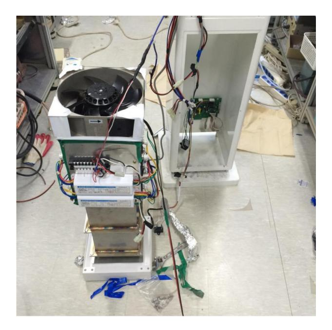
Circulation fan is installed on top of the air cleaning equipment for air circulation inside the equipment. Underneath the fan is a UV lamp that supplies ozone and the nanometer catalyst filter to process pollutants. The circulation fan operates with the capacity of 4 CMM(m3/min) based on the room size of 16.52
