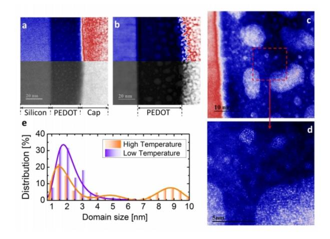
STEM images show cross-sectional views of PEDOT polymers grafted onto substrate material. The material was heated to 100 degrees Celsius (a), and then to 200 degrees C (b). Higher-resoltion views of the high-temperature material (c) and (d) show well-ordered crystallite areas.
