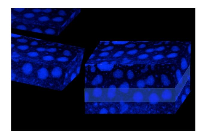
A scanning tunneling electron micrograph (STEM) of the polymer material shows its division into crystalline regions (light areas of orderly dots) and the amorphous, disordered matrix, which is seen as the dark background. The original 2-D STEM views were rendered into 3-D form to create this visualization. Credit: Asli Ugur
