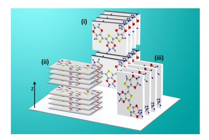
Diagram shows the possible orientations of PEDOT polymer chains relative to a substrate surface (white plane at bottom), in experiments carried out by the MIT team.
