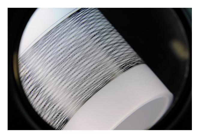
Photograph shows a high strength and high modulus carbon fiber processed at Georgia Tech. Credit: Gary Meek, Georgia Tech
