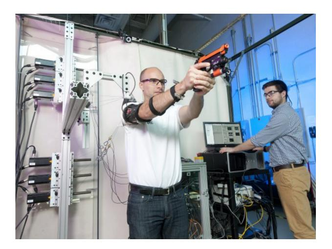
Dan Baechle, left, from the U.S. Army Research Laboratory Multifunctional Materials research team, has created a laboratory prototype of a device he designed to sense and damp out arm tremors for army marksmanship training. Credit: Doug LaFon
