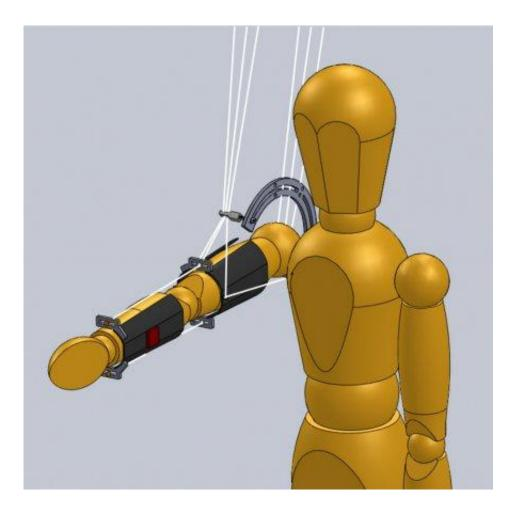
Computer-simulated modeling of the MAXFAS cables, which attach from behind to enable the red sensor to feel and adjust the slightest of arm movement, help the team communicate to human sciences experts the concept of how they would like to improve shooting proficiency. Credit: Doug LaFon
