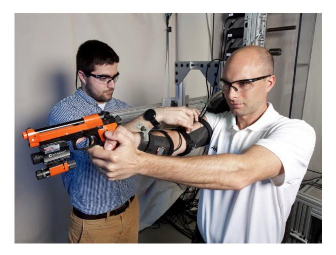
Researchers use high-speed motion sensor OptiTrack cameras mounted around the test area to monitor the mechatronic arm exoskeleton's effect on simulated shooting. Credit: Doug LaFon
