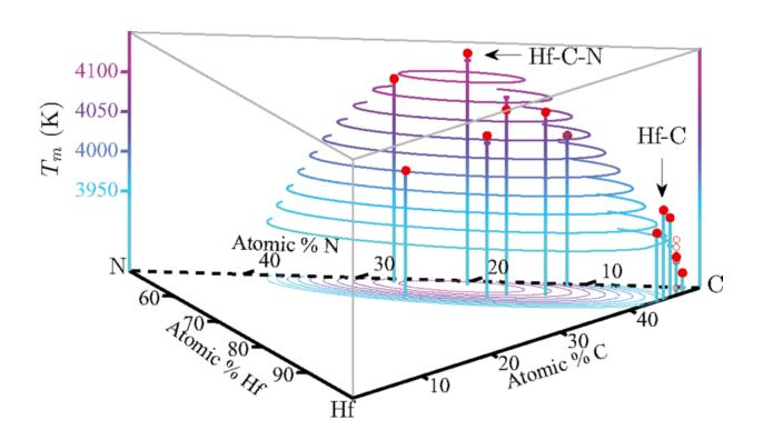
Compounds made from hafnium and carbon have some of the highest known melting points. Using computer simulations, Brown University engineers predict that a material made with hafnium, nitrogen, and carbon will have a higher melting point than any known material. Credit: van de Walle lab / Brown University
