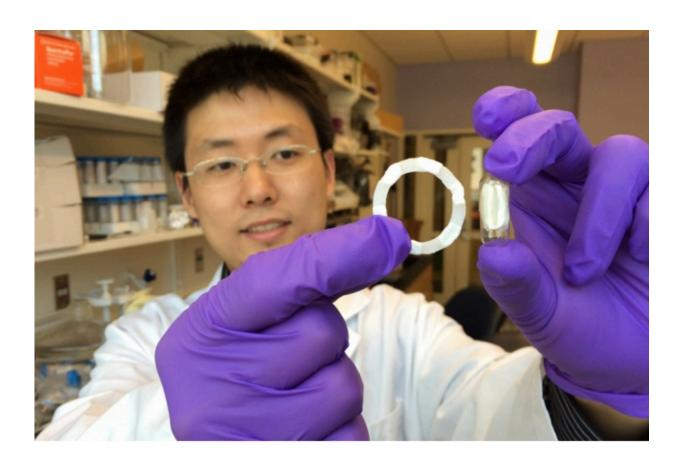
Shiyi Zhang, a postdoc at the Koch Institute and the paper's lead author, holds a ring-shaped device prototype (left), which can be folded into a swallowable capsule (right) for easy and safe oral delivery. Credit: Photo courtesy of the researchers
